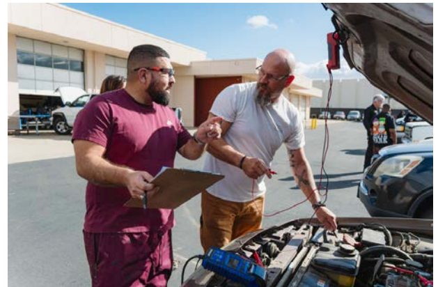
Alejandro and a fellow student performing a battery test.
